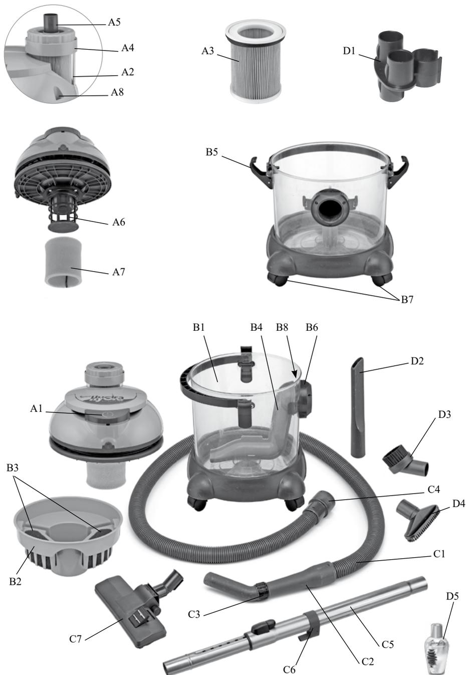
**A. Engine's set.** This section includes an engine, a switch and operating elements. Upper part of this section constitutes HEPA filter used to filter out dust and other small parts from the air that is blown out. Under a foam filter there is a big, plastic float which, as the container fills up, raises and cuts off vacuum at the same time informing about a necessity to empty the container.
